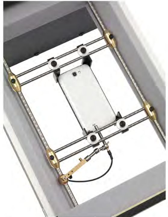
Test jig with DUT and measurement microphone.
